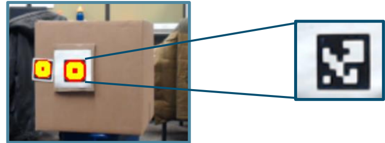
ArUco markers identified by vision system
