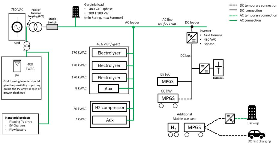
Preliminary architecture design at utility site demonstrating hydrogen asset tie-in to OUC grid
