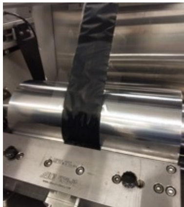
Direct membrane coating with a slot die
