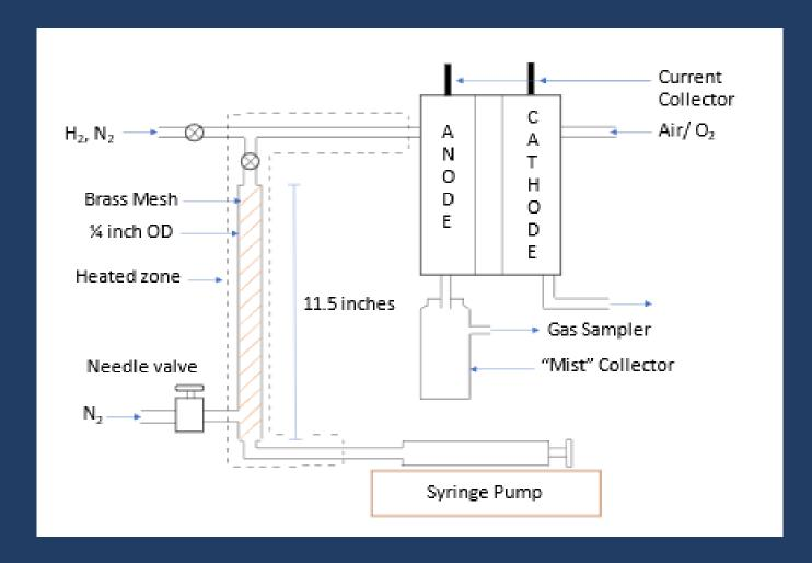
Fuel Cell Apparatus for entering Low-Volatility Liquid Fuels.
