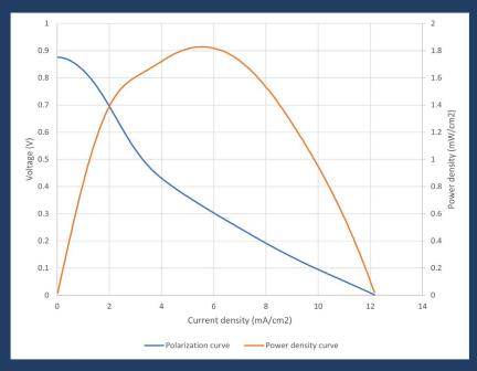
Polarization curve (blue) for cyclohexane. Feed at 0.1 ml/min, vaporized at 160 deg C. Cell at 160 deg C. Scan rate 2mA/sec, sample period 0.5 sec. Max. Power Density (PD): 1.8 mA/cm2
