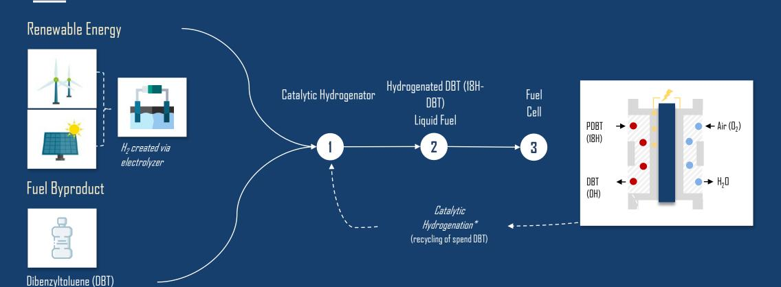
\*Regeneration of "spent" DBT fuel by catalytic hydrogenation demonstrated by Hydrogenious Inc.
