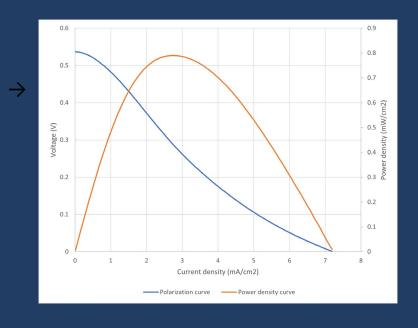
Fuel,0.1ml/min+N2 fed at 200sccm,32psia. Oxygen,200sccm. Scan rate 2mA/sec.
