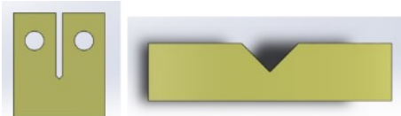
ASTM D5045 Compact Tension & Single Edge Notch Bend
