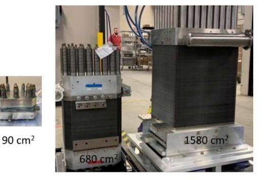
Nel scale up and commercialization: MW stack based on same platform
