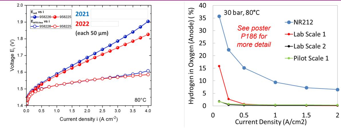
High performance membranes improve overall efficiency Low effective gas crossover at high differential pressure
