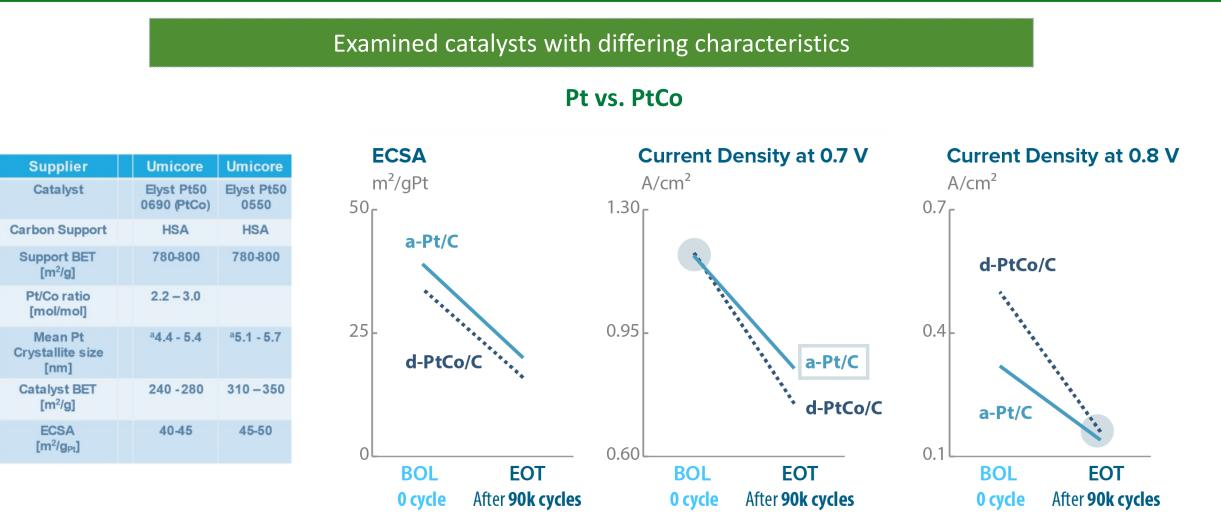
Annealed Pt/C (a-Pt/C) chosen as the baseline to meet durability and current density requirements.
