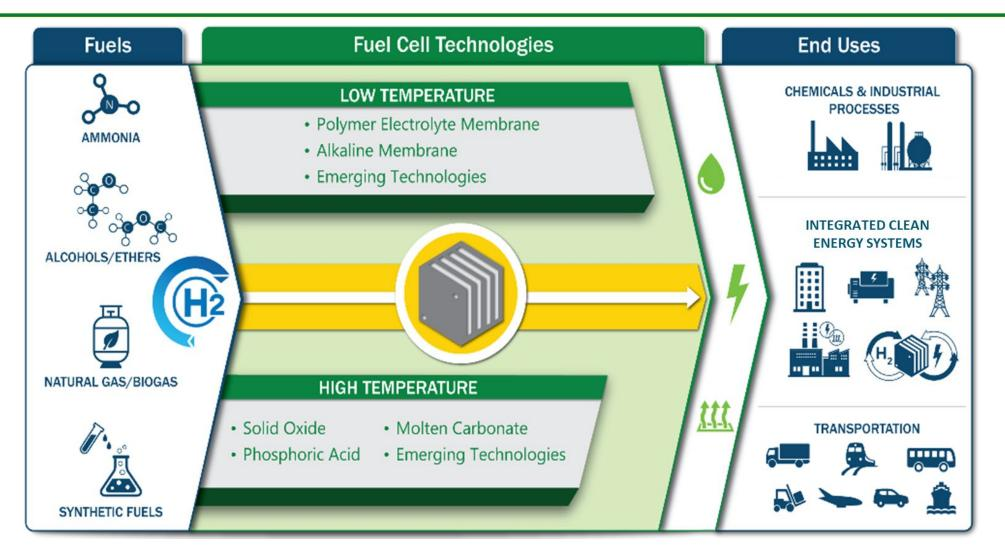
Fuel cells use a wide range of fuels and feedstocks; deliver power for applications across multiple sectors; provide long-duration energy storage for the grid in reversible systems.
