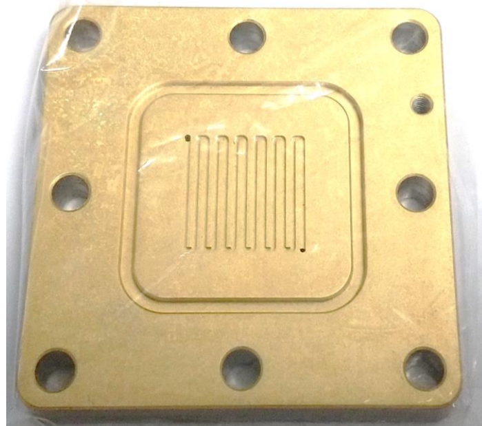
After PVD deposition of ~100 nm thin film Au
