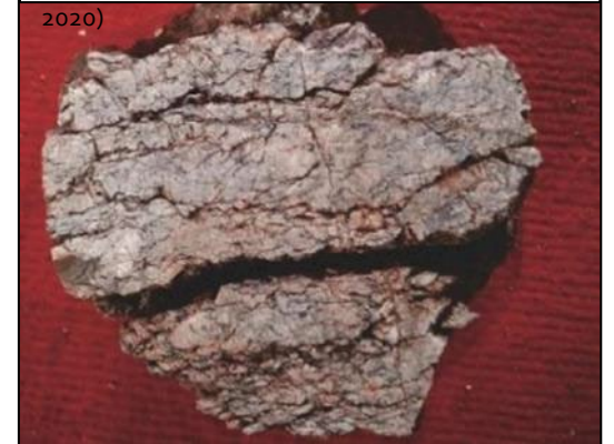
Fractured granite gas reservoir rock from Qaidam Basin, China (Yang et al., 2020)
