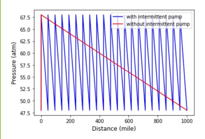
Total NH<sub>3</sub> delivery = 10,000 MT/day= 1000 mile Total pipeline length = 25 °C Pipeline temperature Pipe inlet pressure = 68 atm Pipe outlet pressure =48 atmState = Illinois = 2019 Reference year Pump electricity usage rate = Industrial Each pump rating  $= 300 \, \text{KW}$
