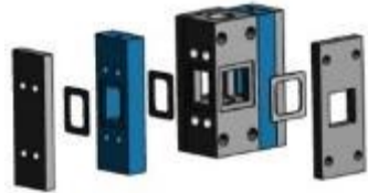
Dual anode cell with high modularity and ease of fabrication
