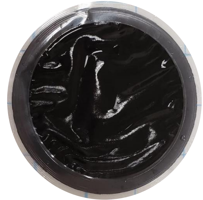
Thrifty CCM Appears Intact After 1000 hr Test
