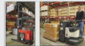
Class-1, -2, and -3 Forklifts Plug Power (GenDrive FCs)
