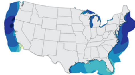
740,000 (kg/km 2 /year) 370,000 <3,000 b) Hydrogen production potential from offshore wind resources, by area
