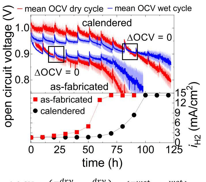
$\Delta OCV = \left(E_{rev}^{dry} - \eta_{ORR}^{dry}\right) - \left(E_{rev}^{wet} - \eta_{ORR}^{wet}\right)$
