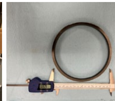
Ring test tooling for fiber strength measurement
