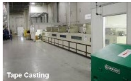
Cell Pilot Manufacturing Processes at VPS: (Tape Casting, Screen Printing, and Co-sintering)
