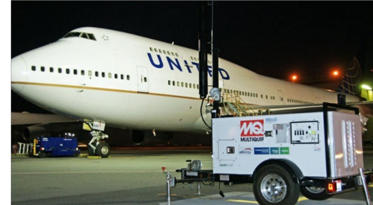
Hydrogen Fuel Cell Mobile Light at the San Francisco International Airport (DOE Project)
