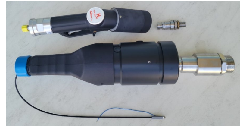
Light Duty WEH nozzle/receptacle (top) compared to Heavy Duty nozzle/receptacle (bottom)
