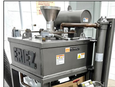
Electromagnetic filter removes iron-rich impurities from graphite flake
