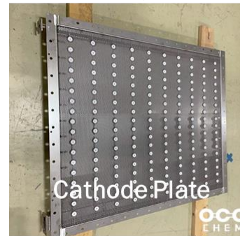
Cathode current collector and GDE support plate with the CO2 flow assembly underneath
