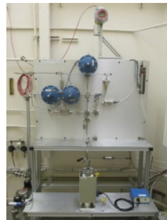
High-pressure hydrogen testing apparatus (Sandia) 5
