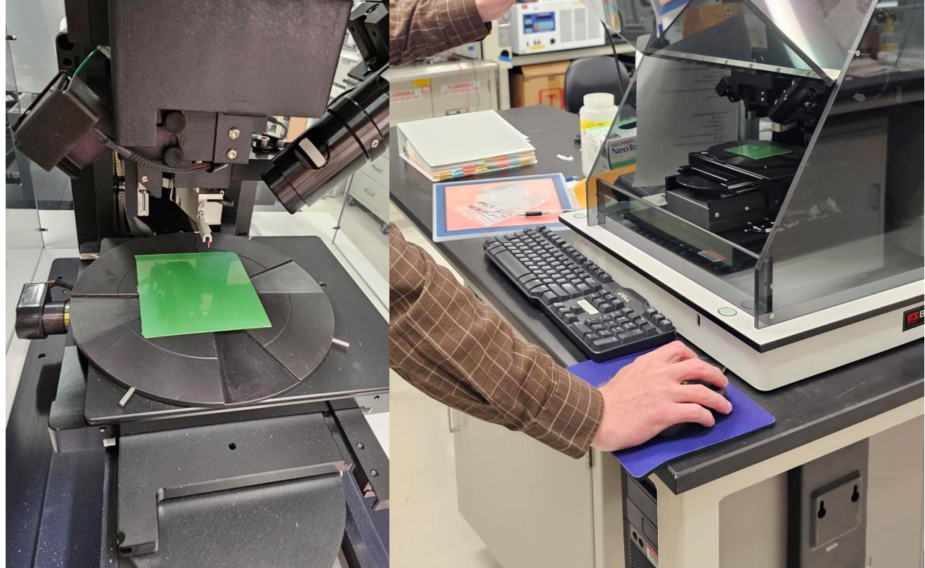
Evaluation of the surface uniformity of the film using a profilometer
