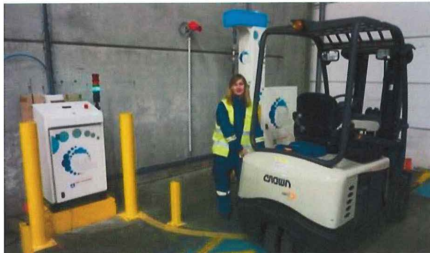
Figure 7. Hydrogen fueling for material handling equipment
