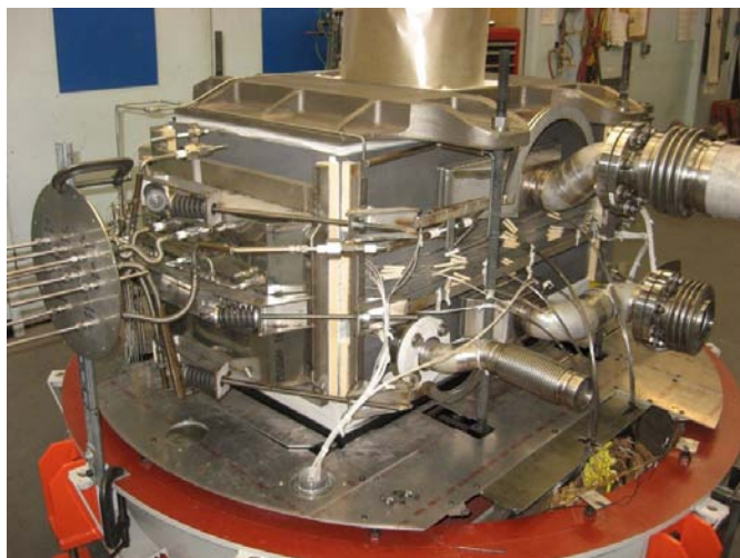
FIGURE 2. A full-area 30 kW technology stack was built for validating selected smart matrix design. The stack was successfully operated for ~6,000 h.
