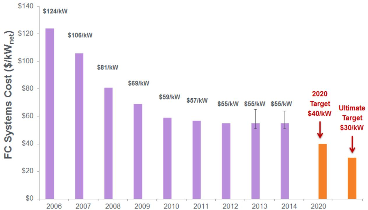
Figure 1. Modeled cost of an 80-kW<sub>net</sub> PEM fuel cell system based on projection to high-volume manufacturing (500,000 units/year). Reported values from 2012 and earlier were adjusted to account for the higher platinum price, the realigned compressor and expander efficiencies, and the Q/ΔT requirement introduced in 2013 (see 2013 cost record).
