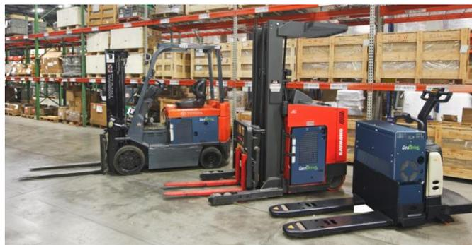
**Figure 4: Fuel Cell Powered Forklifts by Plug Power Inc.**
