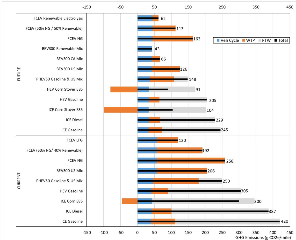
**Figure 2. Life Cycle GHG Emissions (g CO<sub>2e</sub>/mi) for Selected Current (2020) and Future (2050) Fuels and Vehicle Technologies for Small SUVs**
