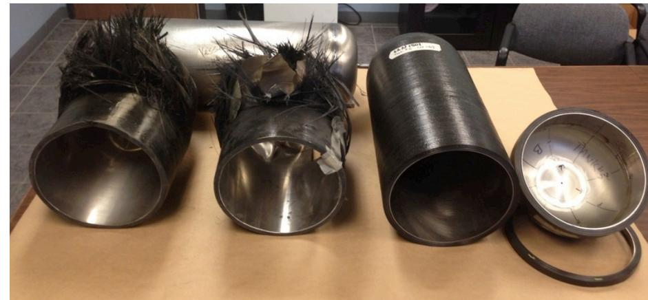
Vessel prototypes have had continuously improving cycle lives. To be soon cryogenically cycle tested
