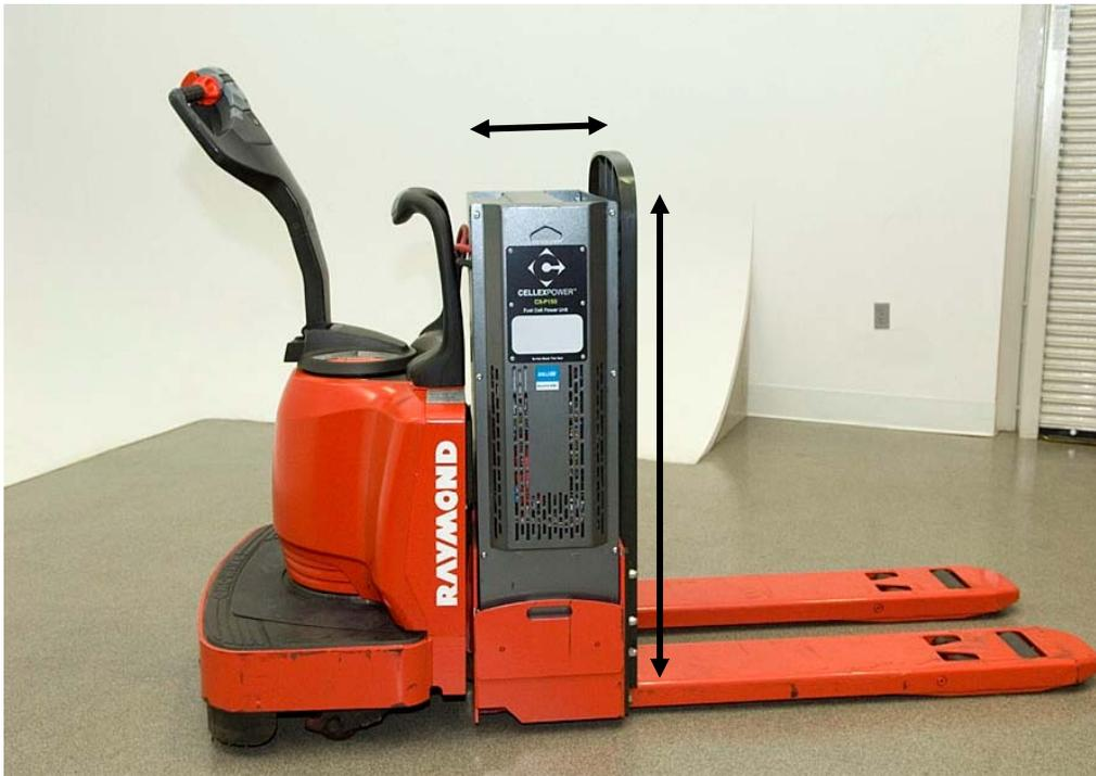
Fuel cell unit in pallet truck
