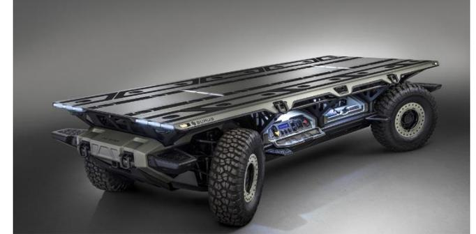
2017 to Present SURUS Fuel Cell Powered Autonomous Vehicle
