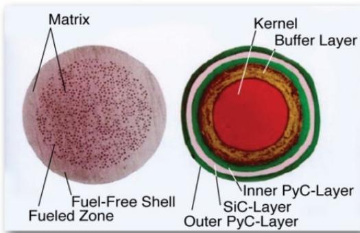
TRISO-coated fuel particles are formed into fuel spheres for pebble bed reactor
