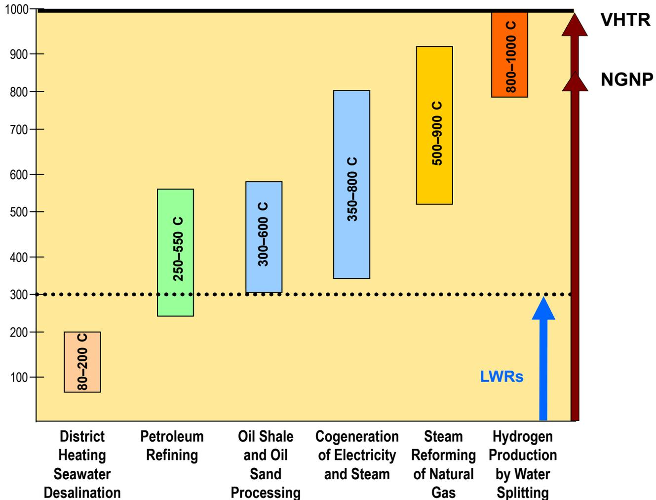
VHTR—Very High Temperature Gas-Cooled Reactors; LWR – Light Water Reactors
