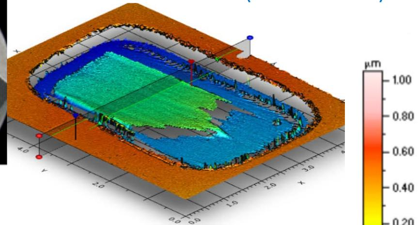
Tandem electrode (p-GaInP<sub>2</sub> on p/n-GaAs) had no detectable etching after 24 hours at about twice the current density
