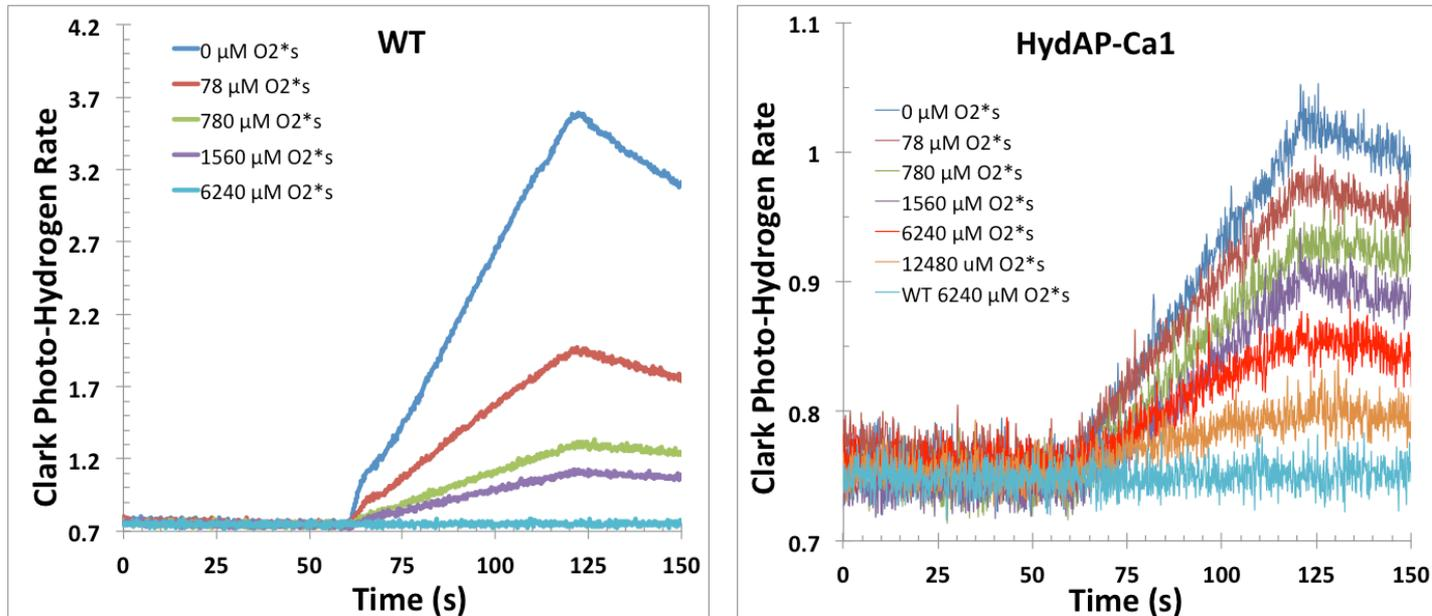
Light-induced H<sub>2</sub> photoproduction by WT and the Ca1 transformant was measured with a Clark electrode, following a 1-min dark incubation in the presence of different amounts of added O<sub>2</sub>. Relative rates are shown above.
