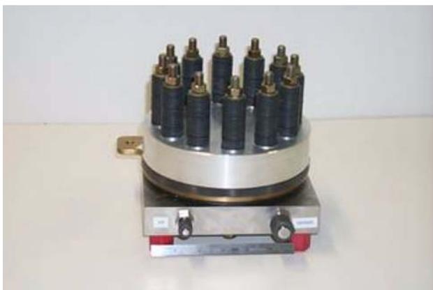
**Figure 4.** Photograph of PES Test Electrolyzer (80 cm<sup>2</sup> Active Cell Area)
