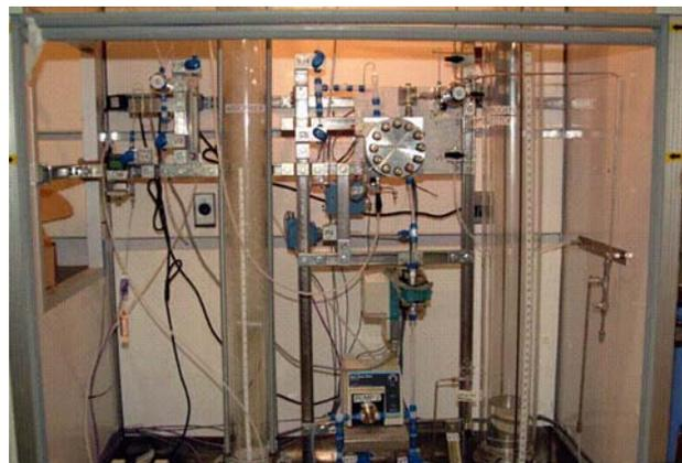
**Figure 3.** SO<sub>2</sub>-Depolarized Electrolyzer Test Facility
