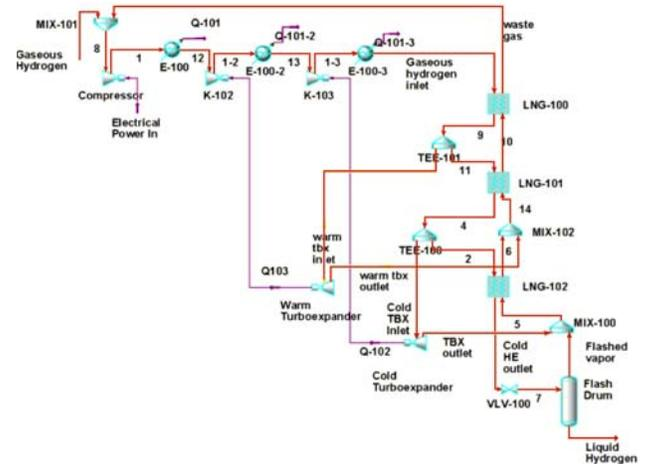
**Figure 3.** Twin Turboexpander-Compressor CRBJT Cycle
