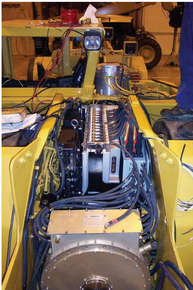
**FIGURE 6.** Traction Motor and Control
