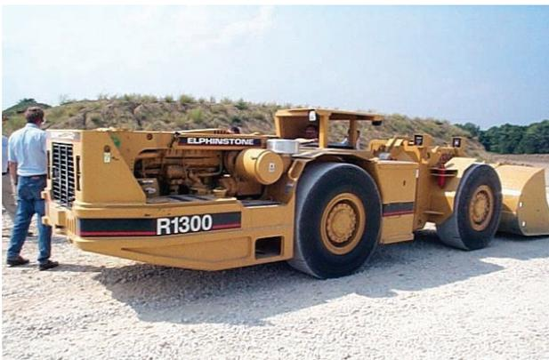
**FIGURE 1.** Diesel-Powered Mine Loader
