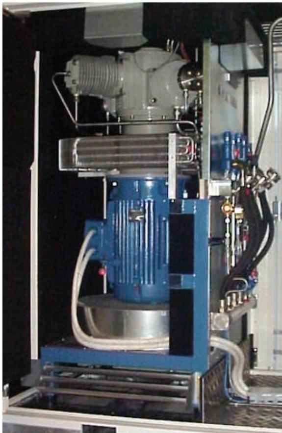
**FIGURE 3.** Novel Multi-Stage Hydrogen Reciprocating Compressor
