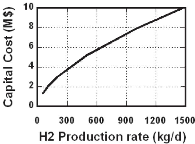
FIGURE 2. Power-law correlation between capital cost for the electrolyzer system and H<sub>2</sub> production rate used in economic analysis to scale the facility to the DOE target size.
