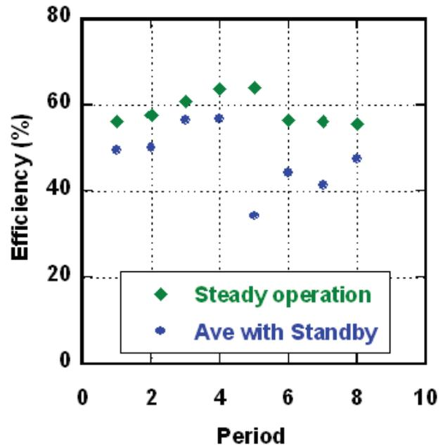
**FIGURE 1.** Efficiency (based on H<sub>2</sub> lower heating value) of the electrolyzer operated at the DTE Hydrogen Technology Park. Circles are monthly averaged performance, including stand-by operation; diamonds are the steady-state operation averaged over periods of at least 10 hours.
