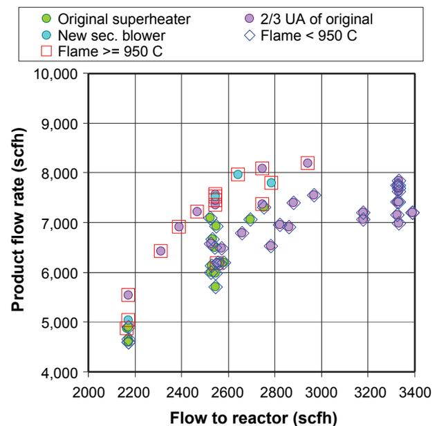
**FIGURE 1.** Hydrogen Production Rate as a Function of NG Flow to the Reformer
