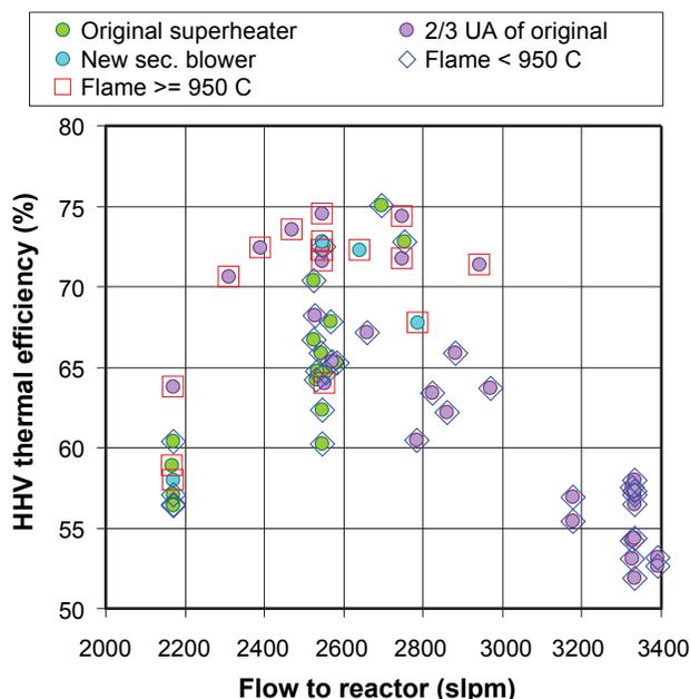
**FIGURE 2.** HHV Thermal Efficiency as a Function of NG Flow to the Reactor
