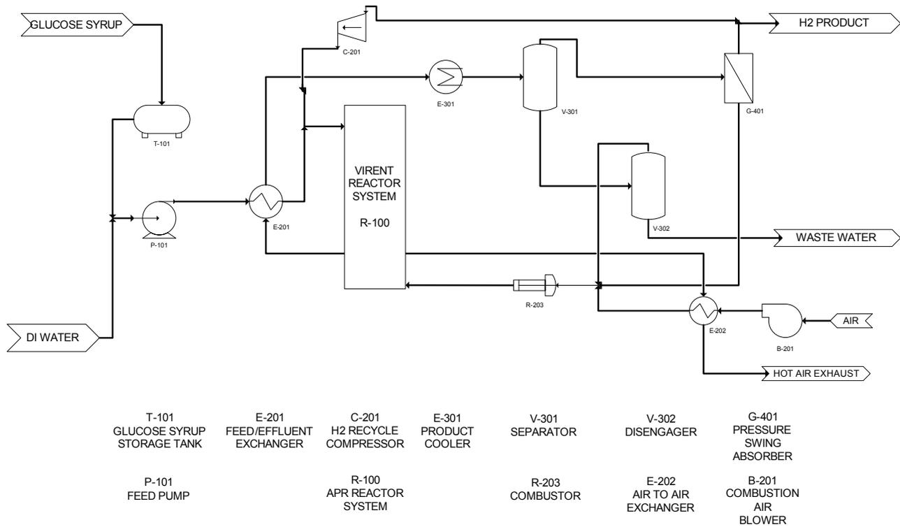
FIGURE 2. PFD of the APR Production Process
