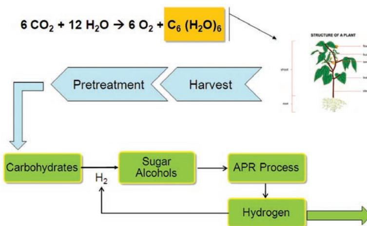
FIGURE 1. Biomass to Hydrogen via the APR Process
