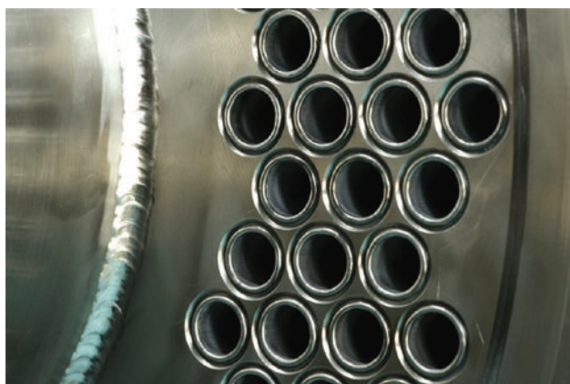
FIGURE 4. AccuSep® tubes welded to tube sheet header using scaled-up process.
