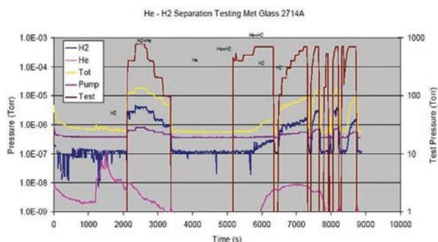
**FIGURE 2.** Preliminary H<sub>2</sub>-He Separations Data for 2714A Metallic Glass Alloys
