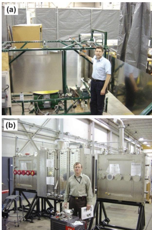
**FIGURE 2.** (a) A roll-to-roll system demonstrating the transport of a 3ft wide web. This web transport system will allow MWOE/Xunlight to deposition thin film Si solar cells on large substrates; and (b) Large area metal sputtering system.
