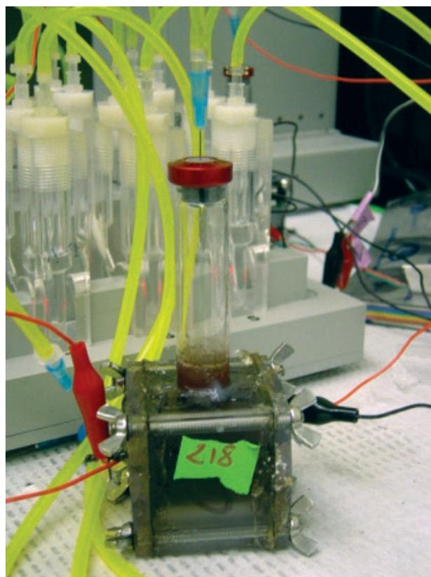
**FIGURE 3.** MEC Reactor used at Pennsylvania State University for Tests
