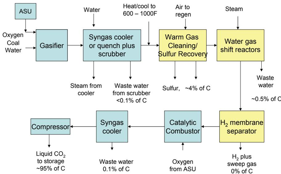
FIGURE 3. Pre-Combustion CO<sub>2</sub> Capture with Eltron Hydrogen Membrane Technology
