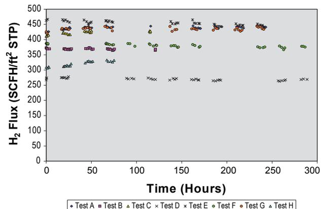
FIGURE 1. Membrane Alloy and Catalyst Alloy Permeation Data
