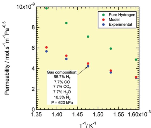
**FIGURE 4.** Comparison of permeability model prediction versus experimental data for a 66.7% H<sub>2</sub>, 7.7% CO, 7.7% CO<sub>2</sub>, 7.7% H<sub>2</sub>O, 10.3% N<sub>2</sub> mixture as a function of temperature. Also shown for reference is the pure hydrogen permeability as a function of temperature.
