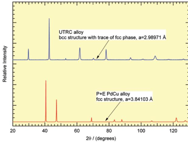
FIGURE 1. X-Ray Diffraction Patterns of Alloy Tube Samples
