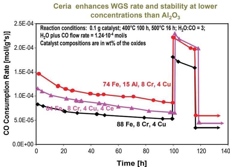
Small amounts of added alumina or ceria produce higher rates and more thermally stable high temperature water gas shift catalysts compared to conventional iron oxide/chromia/copper
