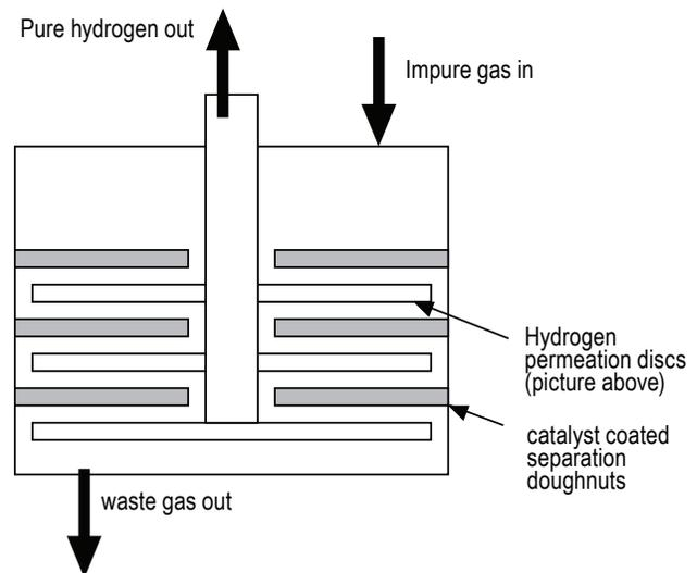
**FIGURE 2.** Schematic of the Disc/Donut Integrated Device Design
