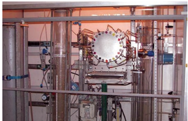
FIGURE 4. Photograph of Multi-Cell SDE Stack Installed in Test Facility
