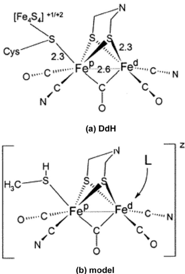
**FIGURE 1.** (a) Active site of the Fe-only hydrogenase, as determined experimentally for *D. desulfuricans*, (b) A model of the  $[2\text{Fe}]_H$  subcluster used in our calculations. A DTN bridging group is assumed.
