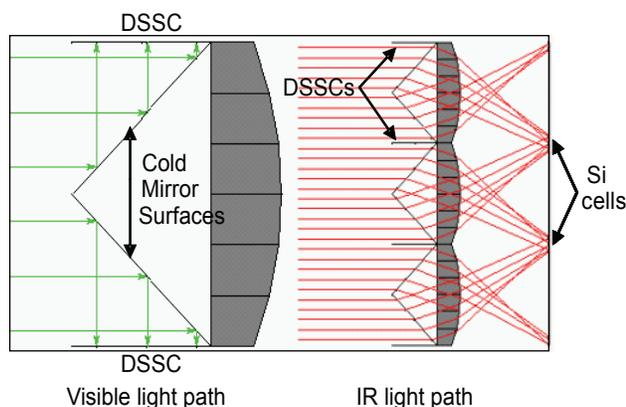
**FIGURE 2.** Ray tracing optical modeling results for a cold mirror-based hybrid DSSC-Si module. The visible light response for one unit cell is shown in the left panel and the right panel shows the IR response and Si cell locations.
