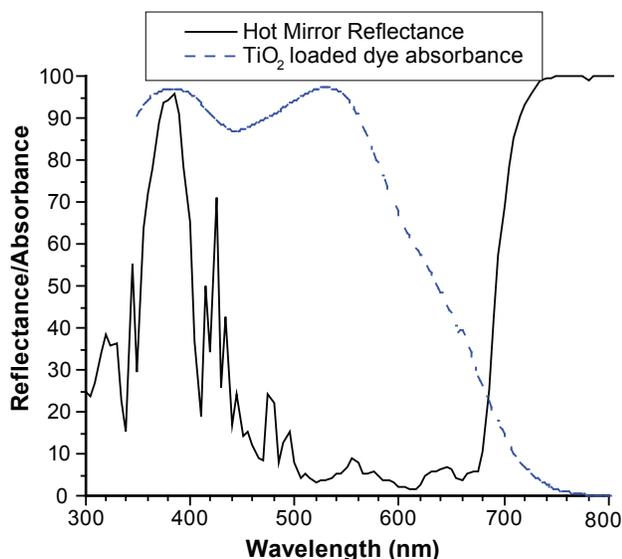
**FIGURE 1.** Hot mirror coated FTO reflectance and absorbance spectrum of a 14  $\mu\text{m}$  N719 dye coated nanoparticulate film as a function of wavelength, showing poor spectral utilization between 600-700 nm.
