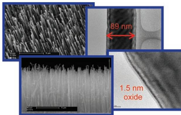
FIGURE 1. p-Si nanowire arrays grown by VLS.
